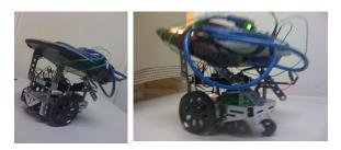
A web-enabled robot prototype, based on the Parallax Boe-Bot robotics kit, with a mounted wireless router and Parallax Internet Net burner Kit (PINK).
