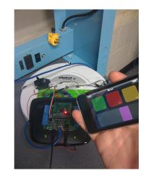
The iRobot with a Linksys wireless router and MAKE controller mounted on it for OSC capability over a Wi-Fi network.
